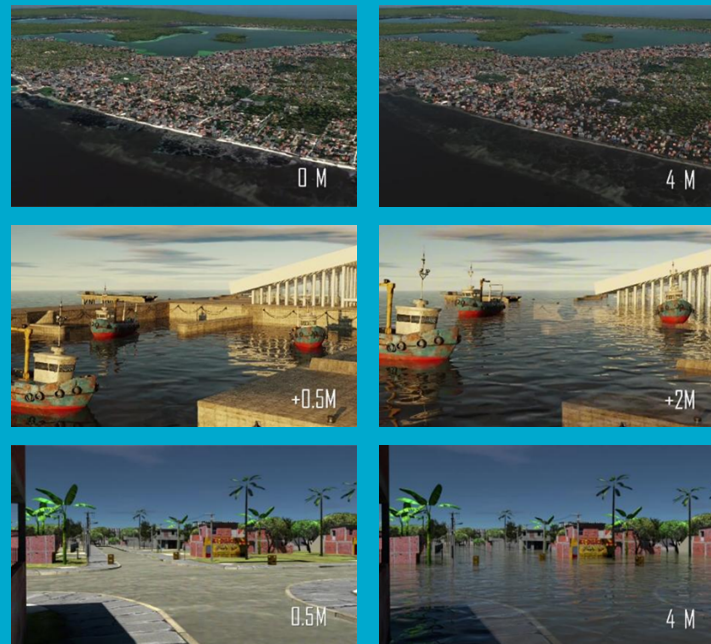
Figure 6. Digital Twin of Tongatapu, allowing sea level rise and flood scenario simulations.
